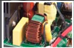
▶ 2 nd stage of transient filtering with ferrite core inductor and X capacitor
