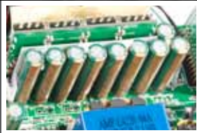
▶ Electrolytic capacitors of DC filtering
