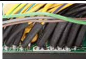
▶ Output rails of 3,3v, 5v, 12v, -12v, 5v with rubber insulation
