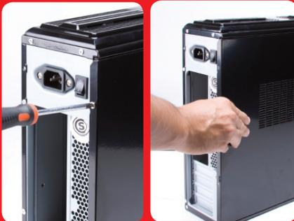
Extract the 4 screws and slide the cover towards the back side of the case. Lift the cover. Remove the two screws and pull the side panel to rear easily way
