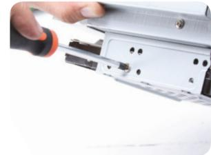
Adjust the screws until the drive is firmly held
