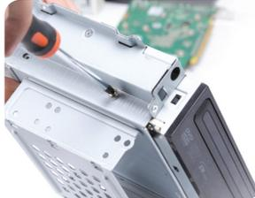
Once the drive has been placed, match its holes with the ones in the chassis structure.
