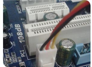
3-pin connector available to connect to 3-pin male connector of motherboard.
