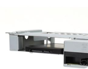
Insert 2.5" SSD driver in the corresponding bay as shown in the picture.
