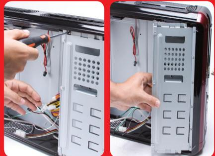
To remove the multi-bay tray, unscrew it from the chassis and lift up. Remove the screws to release the Multibay.
