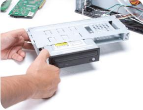
Withdraw the multi-bay tray from the case and insert the optic drive in the corresponding bay.
