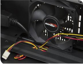
Top fan cooler with 3-pin female connector
