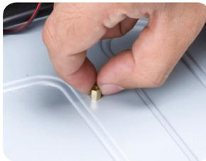
Use the bronze screws over the plating of the chassis.
