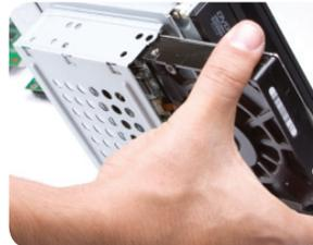
Insert the optical drive in the corresponding bay.
